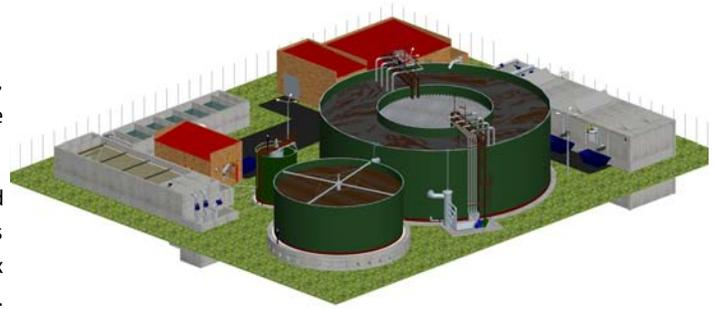
Fig.3. Baghdad Wastewater Treatment plant final 3D Detailed Engineering plot.
