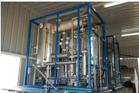
Fig. 2. Two industrial three component continuous distillation units for biodiesel.
